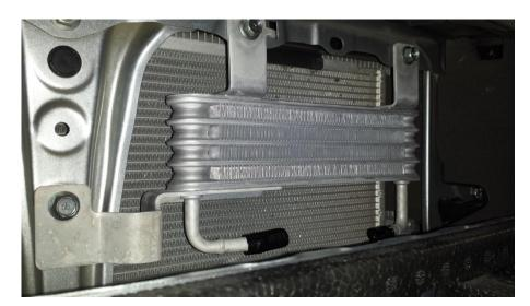
4. Attach the CVT cooler Hoses with 2 of the clamps to the CVT Cooler, run through existing hose holder in foam panel next to the drivers headlight and position them into engine compartment area under the headlight.
